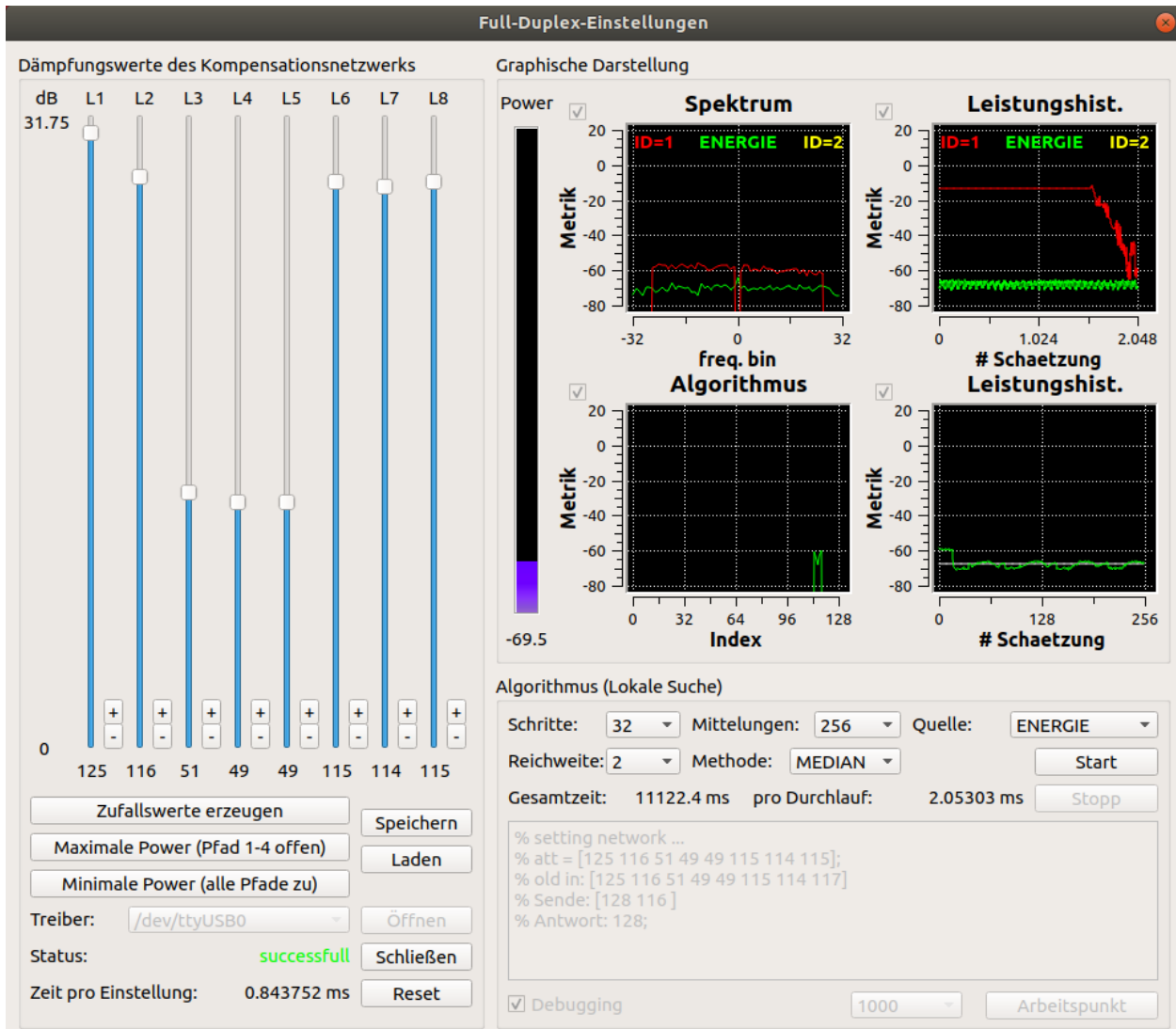
Figure 10: Initial Compensation of Self-Interference (Red Curves; ID = 1).
