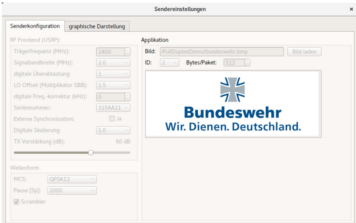
Figure 11: TX Configuration with the Chosen Picture to be Transmitted.
